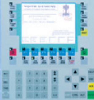
The Thyricon excitation system controller is a user-friendly Human Machine Interface (HMI).
