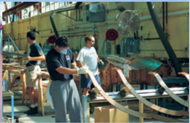
Stator bar manufacturing in Mississauga
